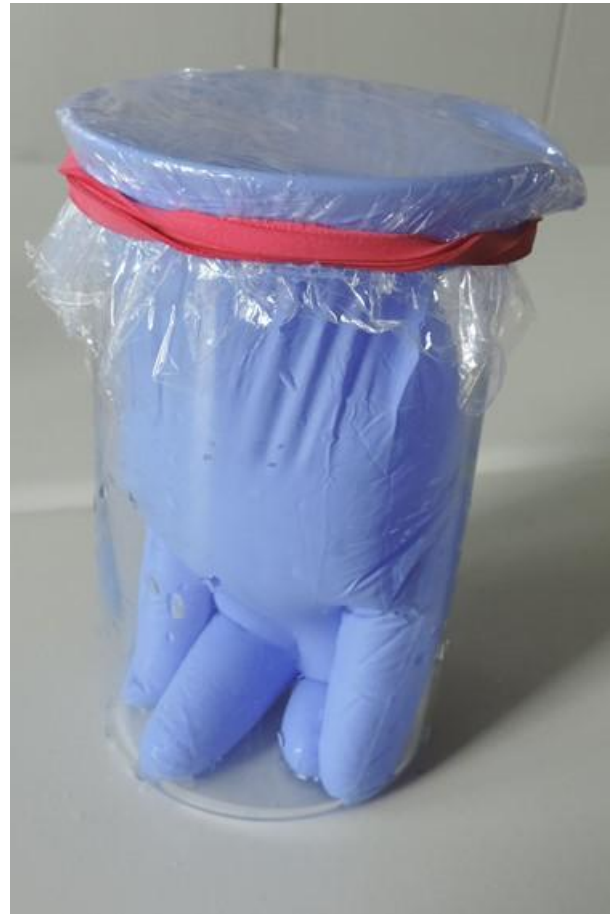
Fig. 2: Glove, filled and pulled over a beaker; covered with film
